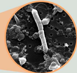
Swollen Cloud Nine halloysite tubes and kaolinite plates after carbon capture
